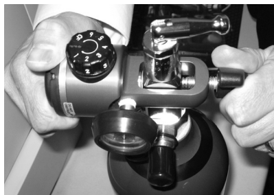
FIGURE 3.1 Attaching the IOC100P to the Cylinder
